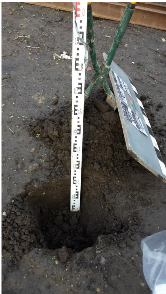
Photograph E: Location V6. Soil well in excess of 300mm
